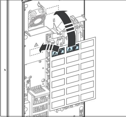
3. For frames R6 and R8: Remove the shroud on the power cable terminals,
