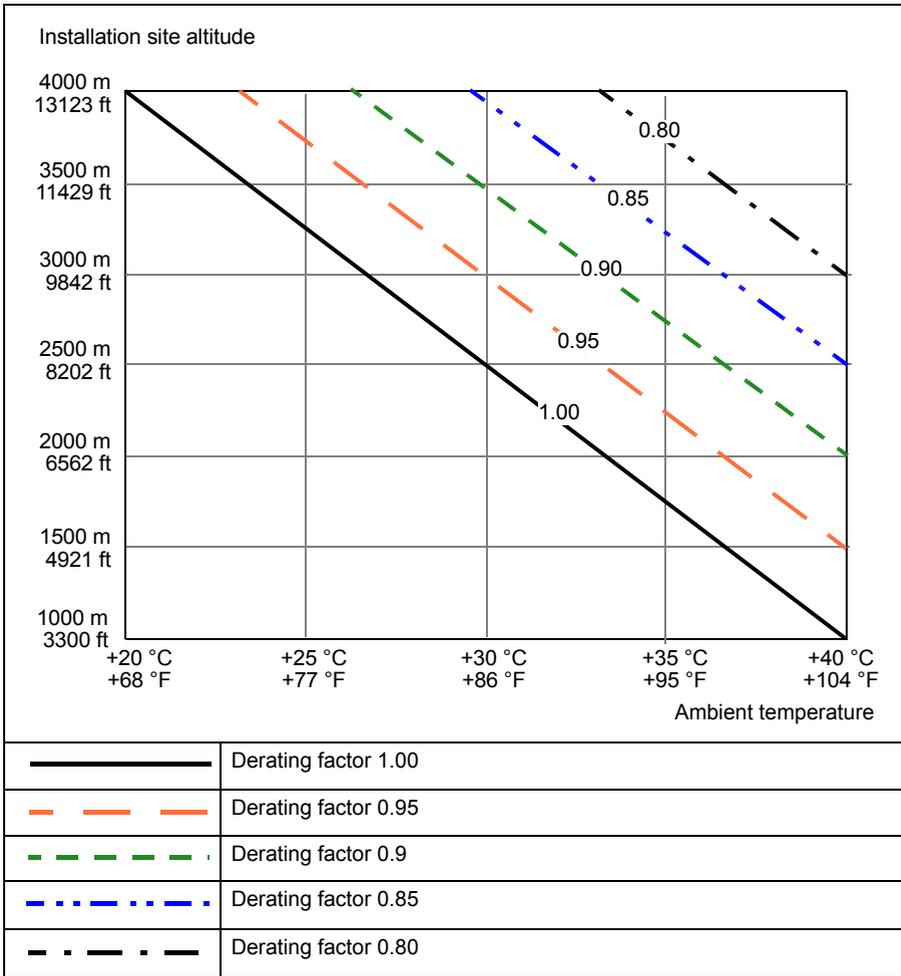
The altitude derating can be reduced if the temperature is below +40 °C, for example, if the temperature is 30 °C, the derating factor is  $1 - 1.5\% \cdot 10 = 0.85$ . You can reduce the output current by 35% instead of 40% at 4000 meter above the sea level.
