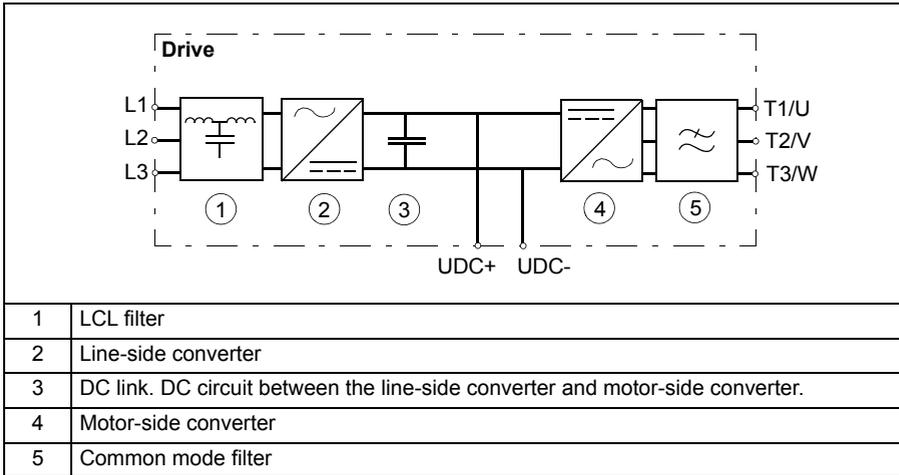
The line-side converter rectifies three phase AC current to direct current for the intermediate DC link of the drive. The intermediate DC link further supplies the motor-side converter that runs the motor.
