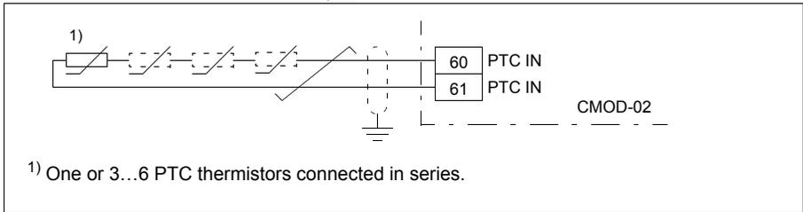
The PTC input is reinforced/double insulated. If the motor part of the PTC sensor and wiring are reinforced/double insulated, voltages on the PTC wiring are within SELV limits.
