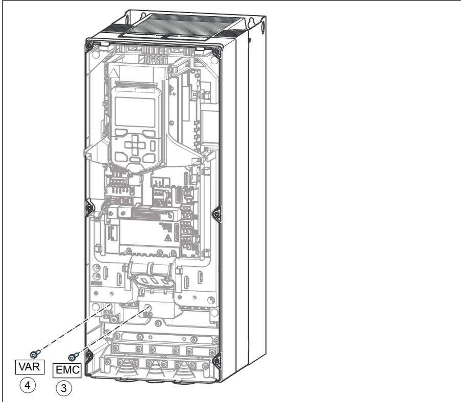
■ **Disconnecting internal EMC filter and ground-to-phase varistor – frame R6**
