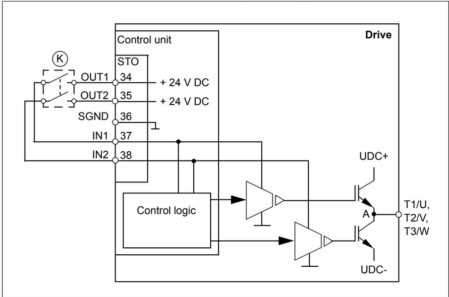
■ Connection with external +24 V DC power supply
