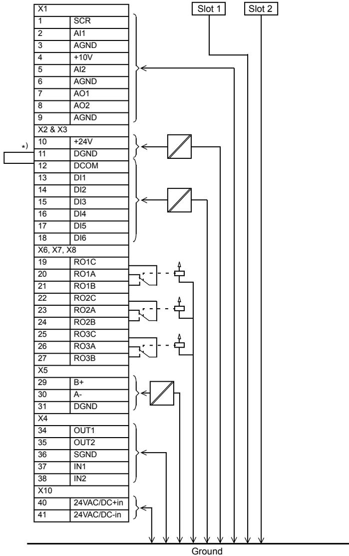
\*) Jumper installed at factory
