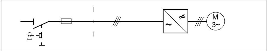
Size the fuses at the distribution board according to instructions given in chapter [Technical data](#). The fuses will protect the input cable in short-circuit situations, restrict drive damage and prevent damage to adjoining equipment in case of a short-circuit inside the drive.
