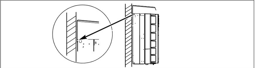
6. Tighten the bolts in the wall securely.
