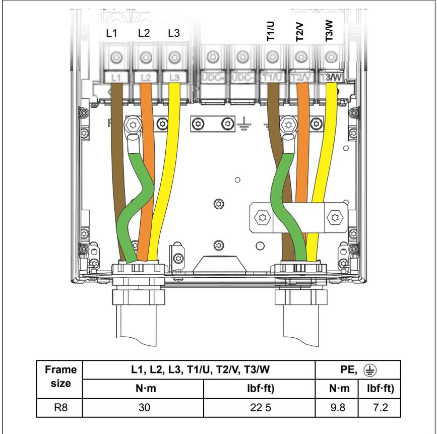
**Note 1 for frame R8:** Install the side plates if removed.
