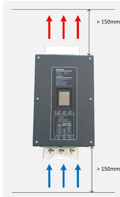
Figure 9 – Air flow around the soft starter
