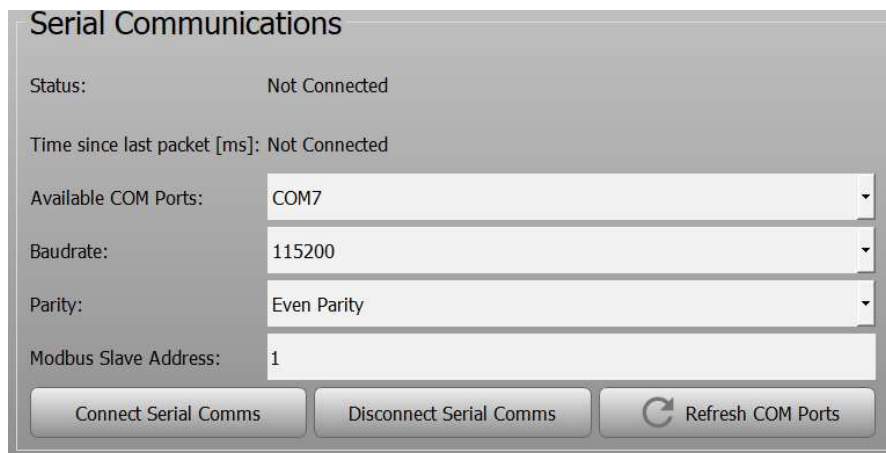
Figure 48 – MEssoftstart PC Application detects the COM port of the Modbus-USB cable
