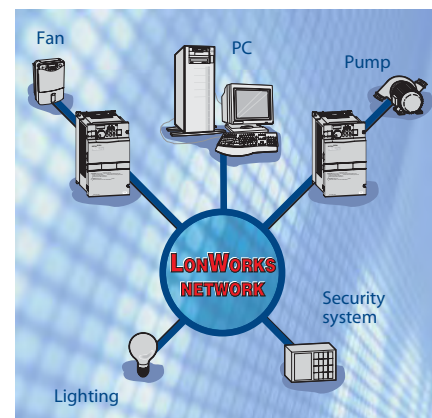
The FR-F740/F746 in a LonWorks network system
